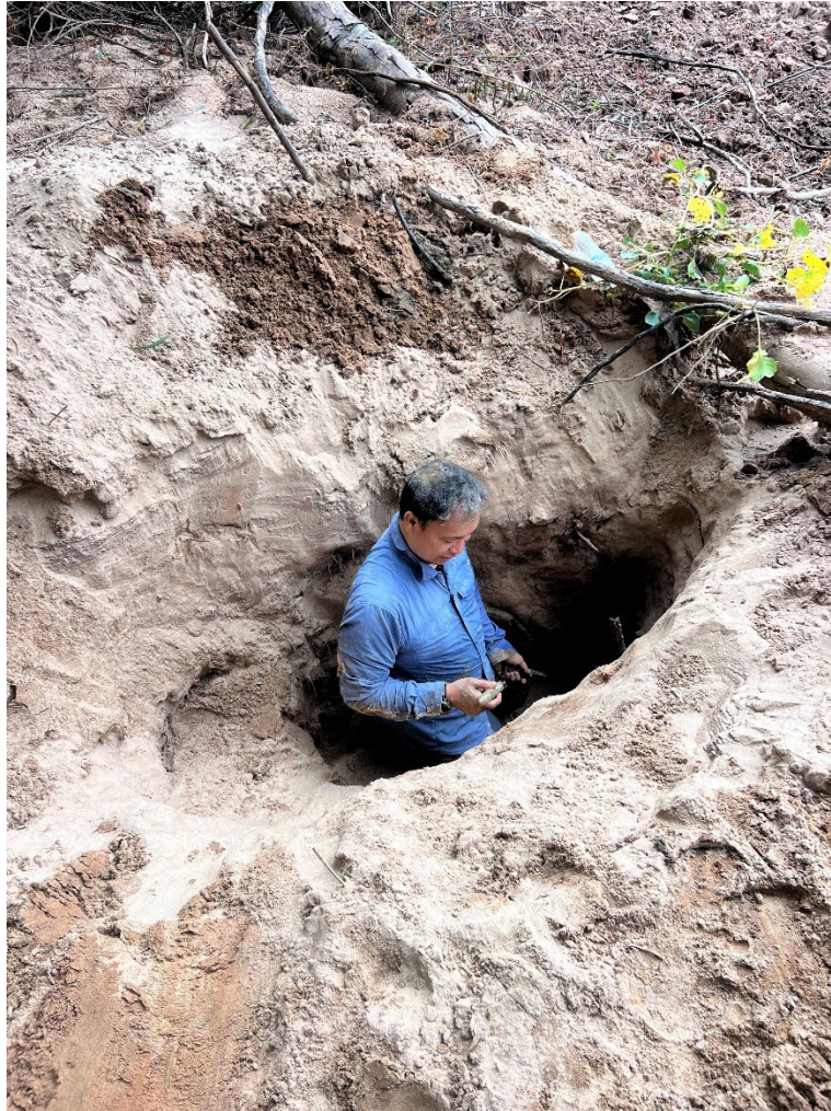
Figure 4.2 Recovery of a pressure transducer following flooding on the Brazos River using a metal detector and a spade.
