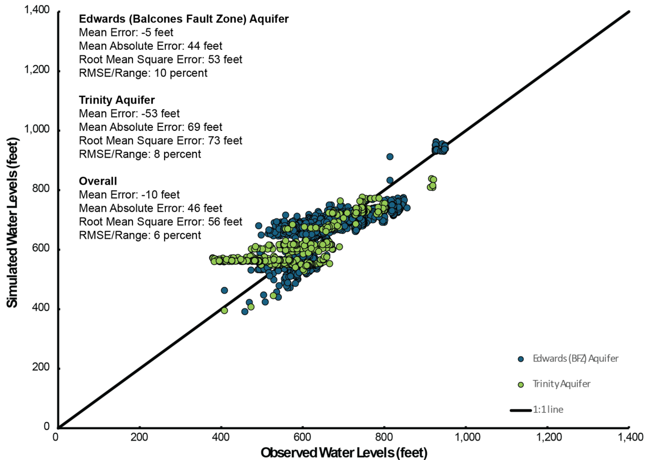
Figure 3.2.2. Cross plot of measured and simulated water levels for the northern segment of the Edwards (Balcones Fault Zone) Aquifer (Layer 1) and the Trinity Aquifer (Layer 3).
