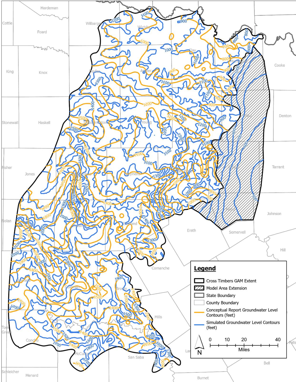
Figure 4-33. Simulated groundwater level contours as compared to interpolated measured groundwater level contours from the conceptual model.
