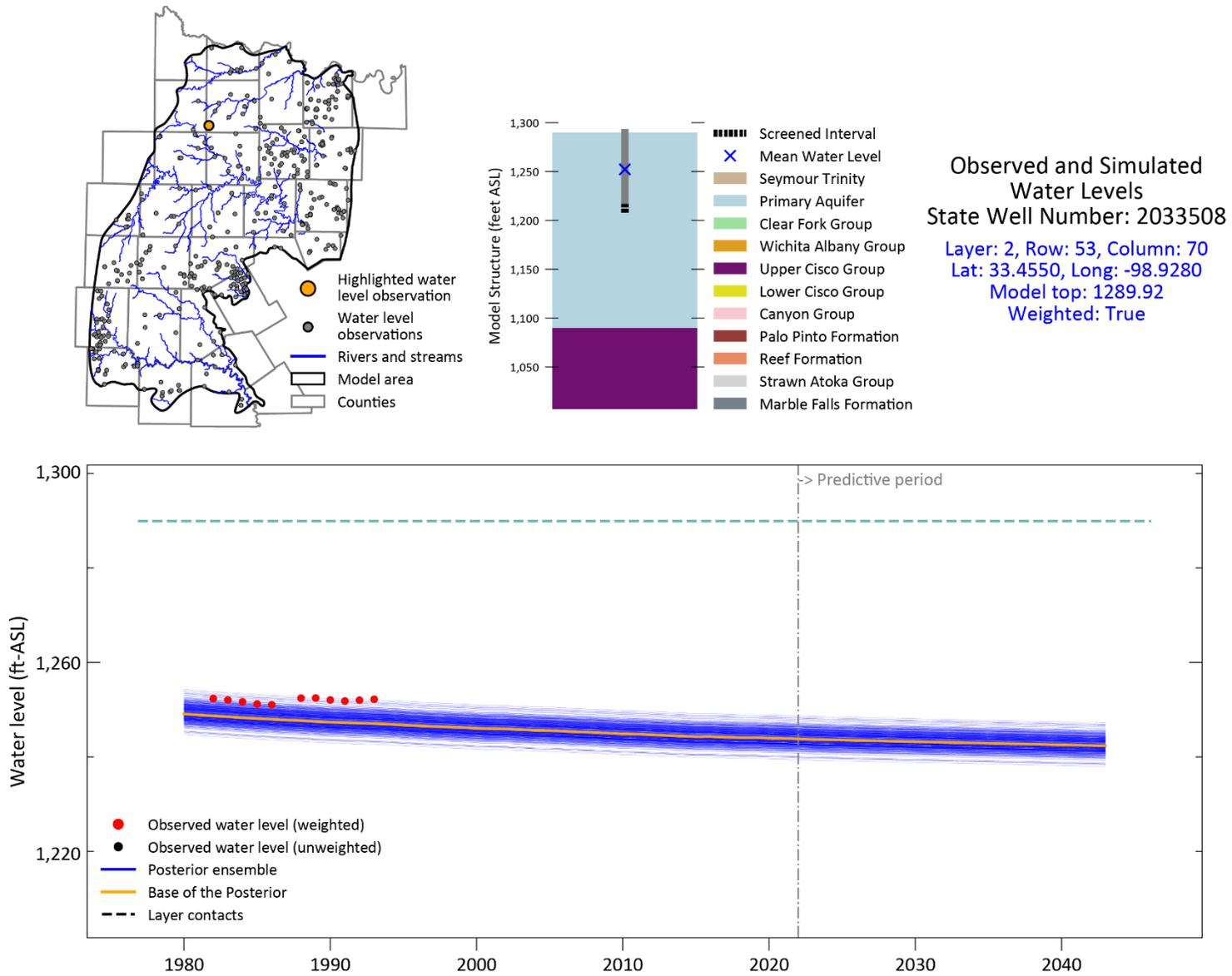
Figure 4-36. Observed (red dots) and simulated (blue lines) groundwater levels in State Well Number 2033508.
