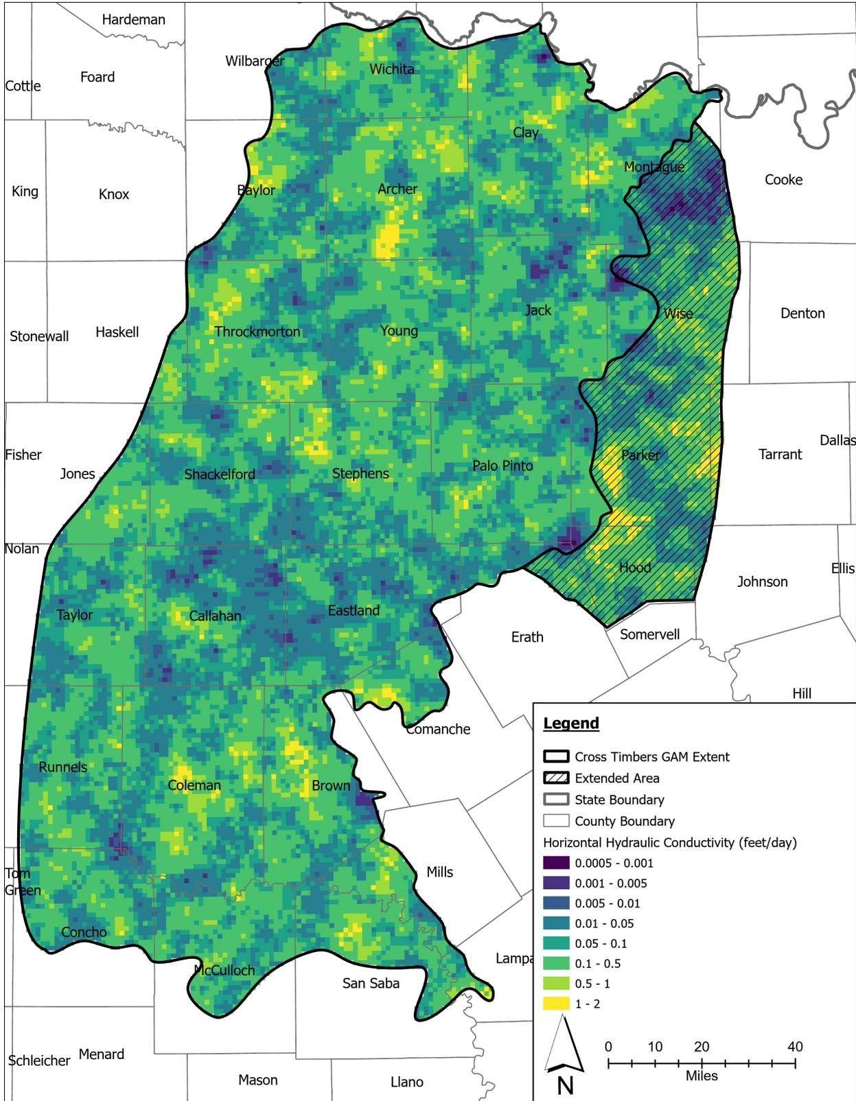
Figure 4-10. Calibrated horizontal hydraulic conductivity for Layer 2.
