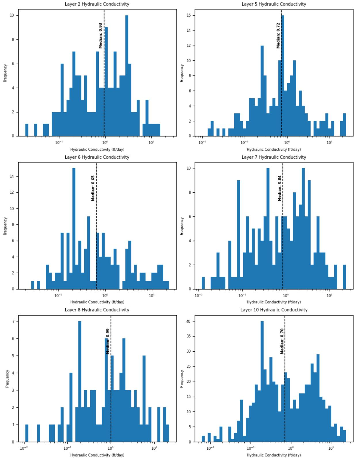
Figure 4-2. Histograms of measured hydraulic conductivity by model layer.
