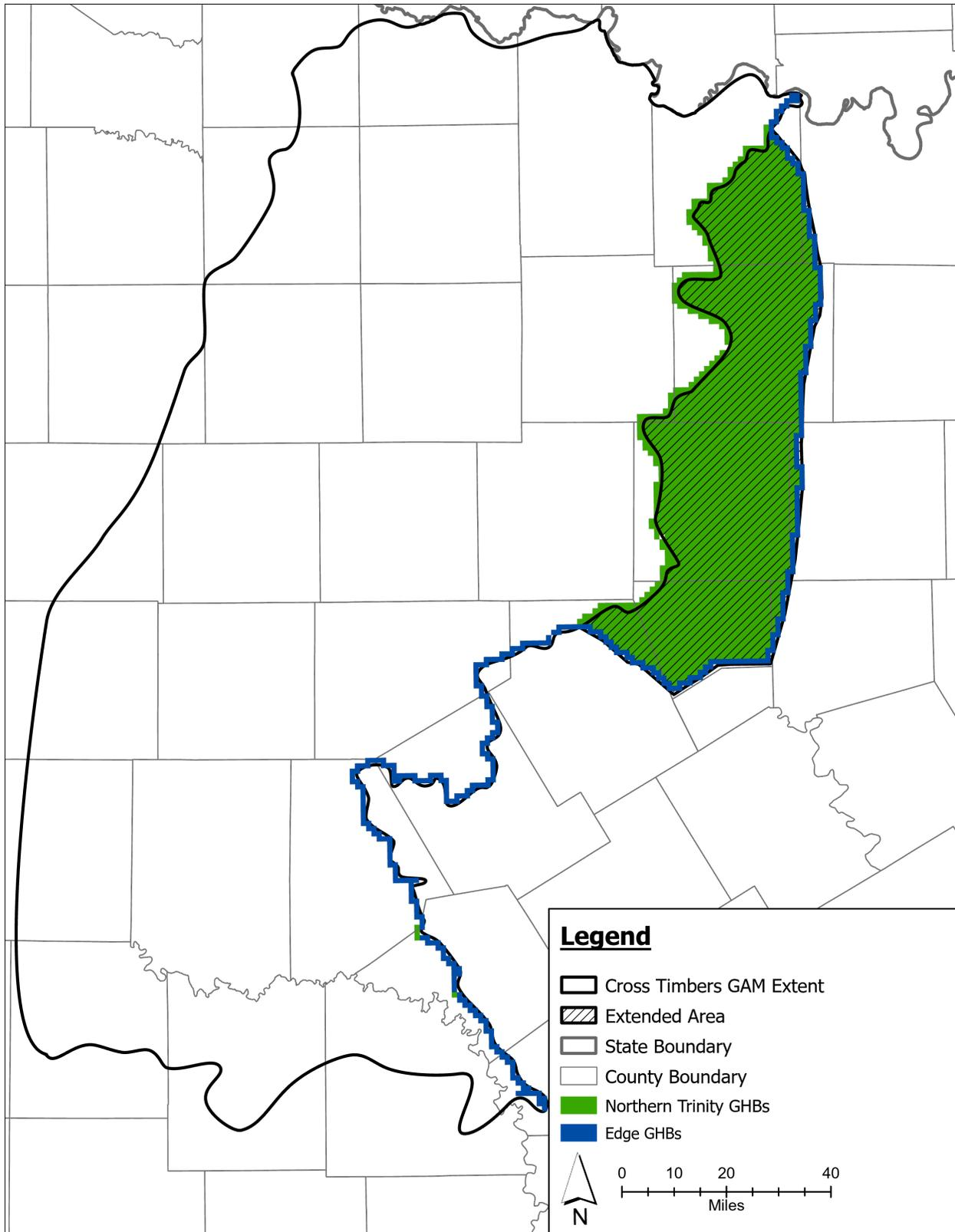
Figure 3-21. General head boundary cells for edge cells and Northern Trinity Aquifer in the extended area.
