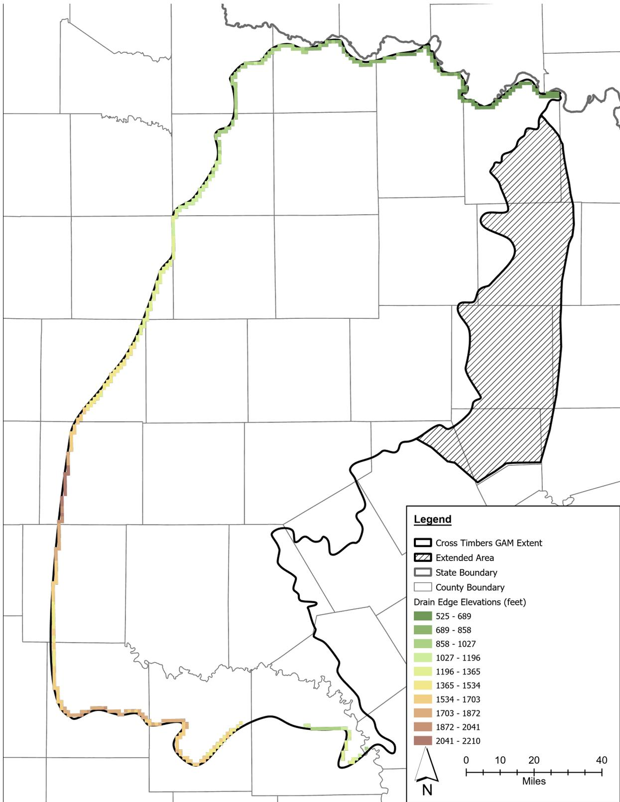
**Figure 3-20. Locations and elevations of edge drain cells.**
