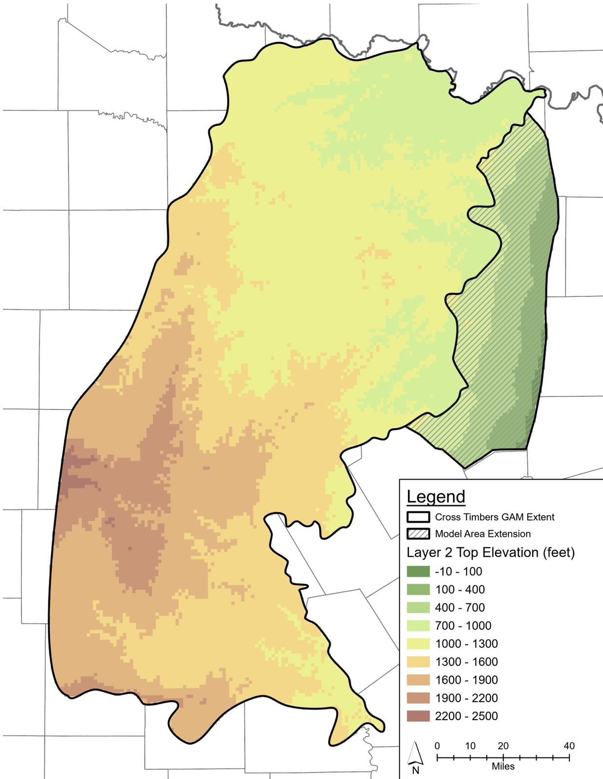
Figure 3-2. Top elevation of Layer 2, primary aquifer, non-shaded areas within the GAM Extent represent inactive and/or vertical pass-through cells.
