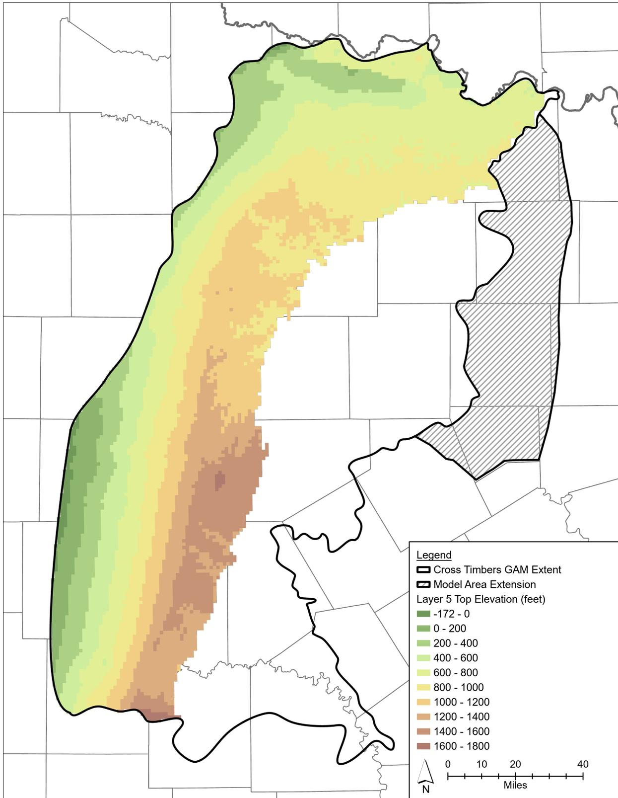
Figure 3-5. Top elevation of Layer 5, Upper Cisco Group, non-shaded areas within the GAM Extent represent inactive and/or vertical pass-through cells.
