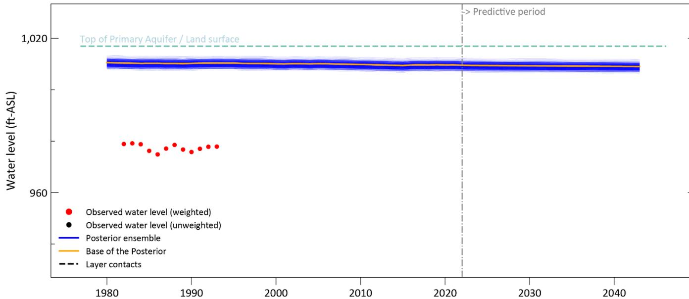
Figure 4-39. Observed (red dots) and simulated (blue lines) groundwater levels in State Well Number 2038403.
