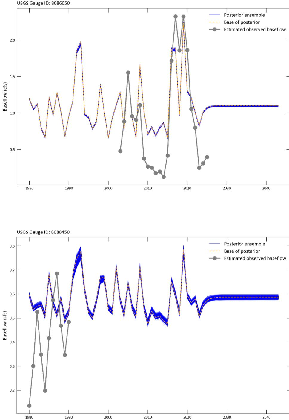
Figure 4-43. Observed (gray line with dots) and simulated (blue lines) baseflow at United States Geological Survey gauge stations 8086050 and 8088450. The base of the posterior is shown in orange.
