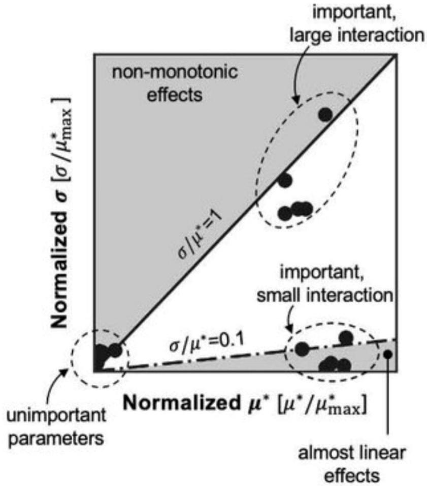
Figure 5-1. Conceptual figure for interpreting parameter sensitivity.
