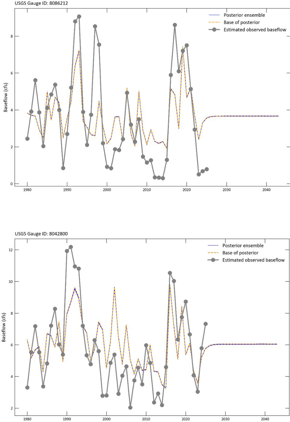
**Figure 4-40. Observed (gray line with dots) and simulated (blue lines) baseflow at United States Geological Survey gauge stations 8086212 and 8042800. The base of the posterior is shown in orange.**
