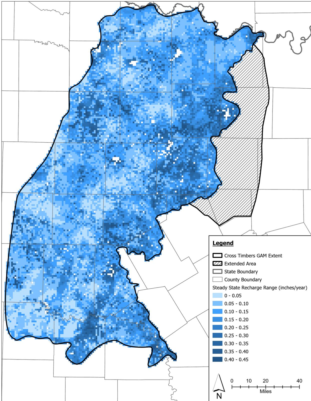
Figure 4-13. Calibrated steady-state recharge rate map.
