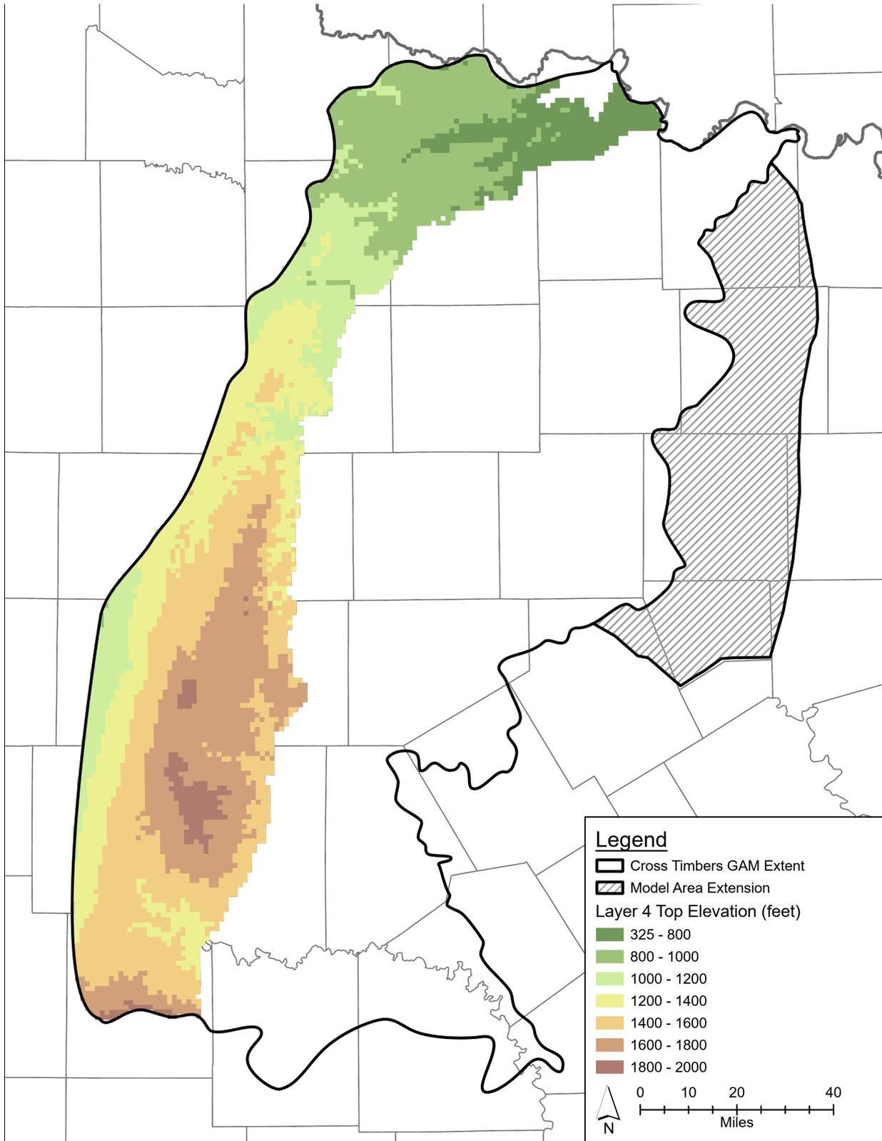
**Figure 3-4. Top elevation of Layer 4, Wichita-Albany Group, non-shaded areas within the GAM Extent represent inactive and/or vertical pass-through cells.**
