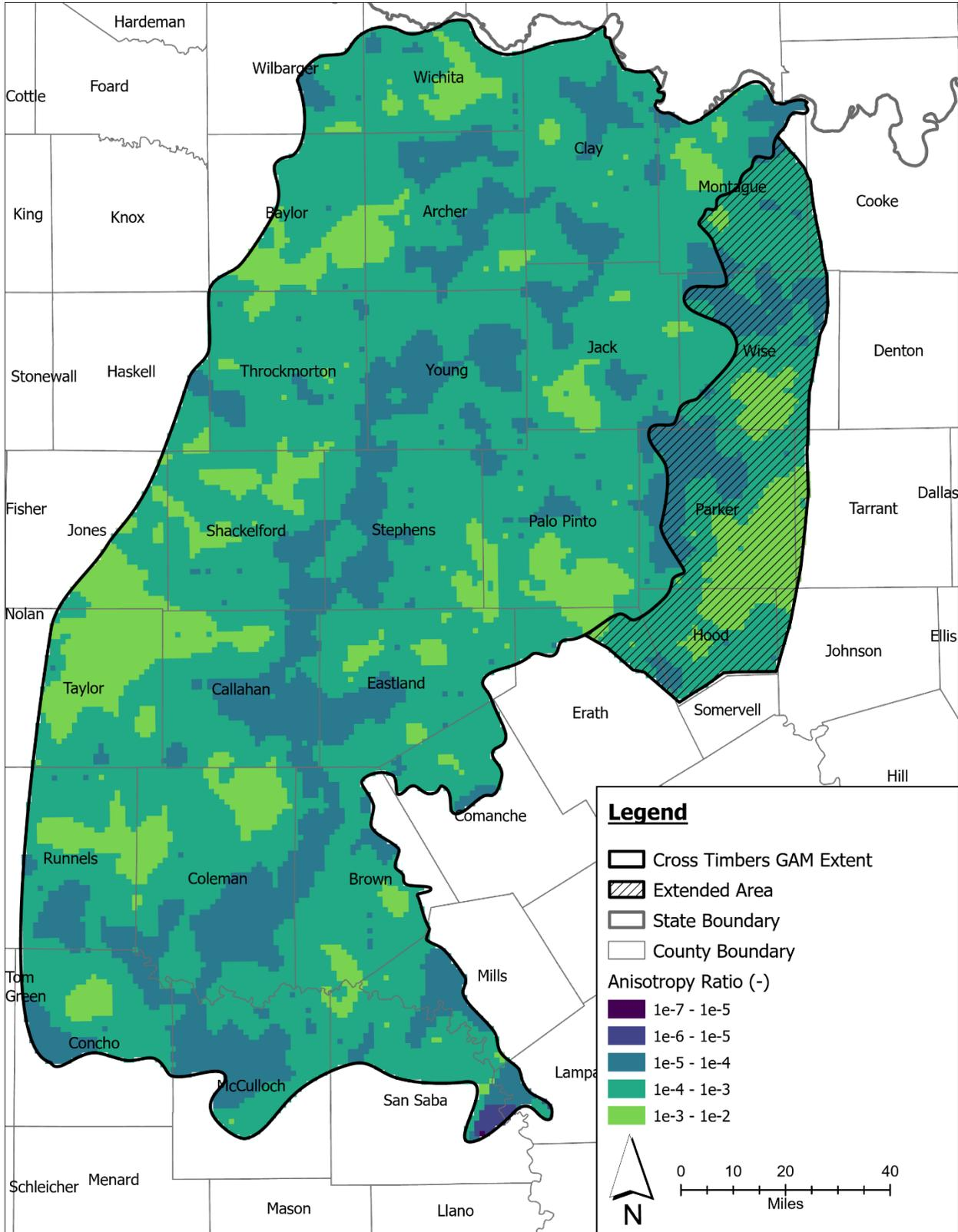
Figure 4-11. Calibrated vertical anisotropy ratio for Layer 2.
