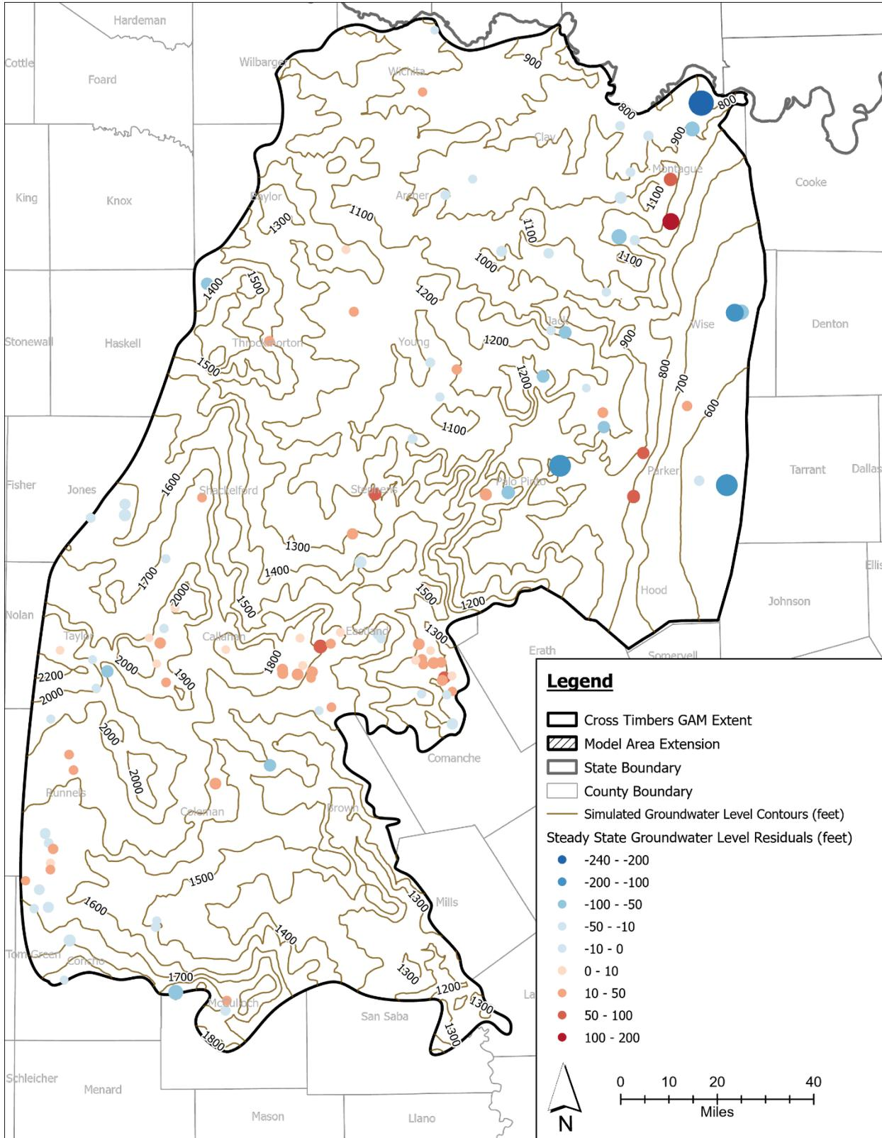
Figure 4-31. Steady state groundwater level residuals (observed minus simulated) in the primary aquifer and simulated steady state groundwater level contours.
