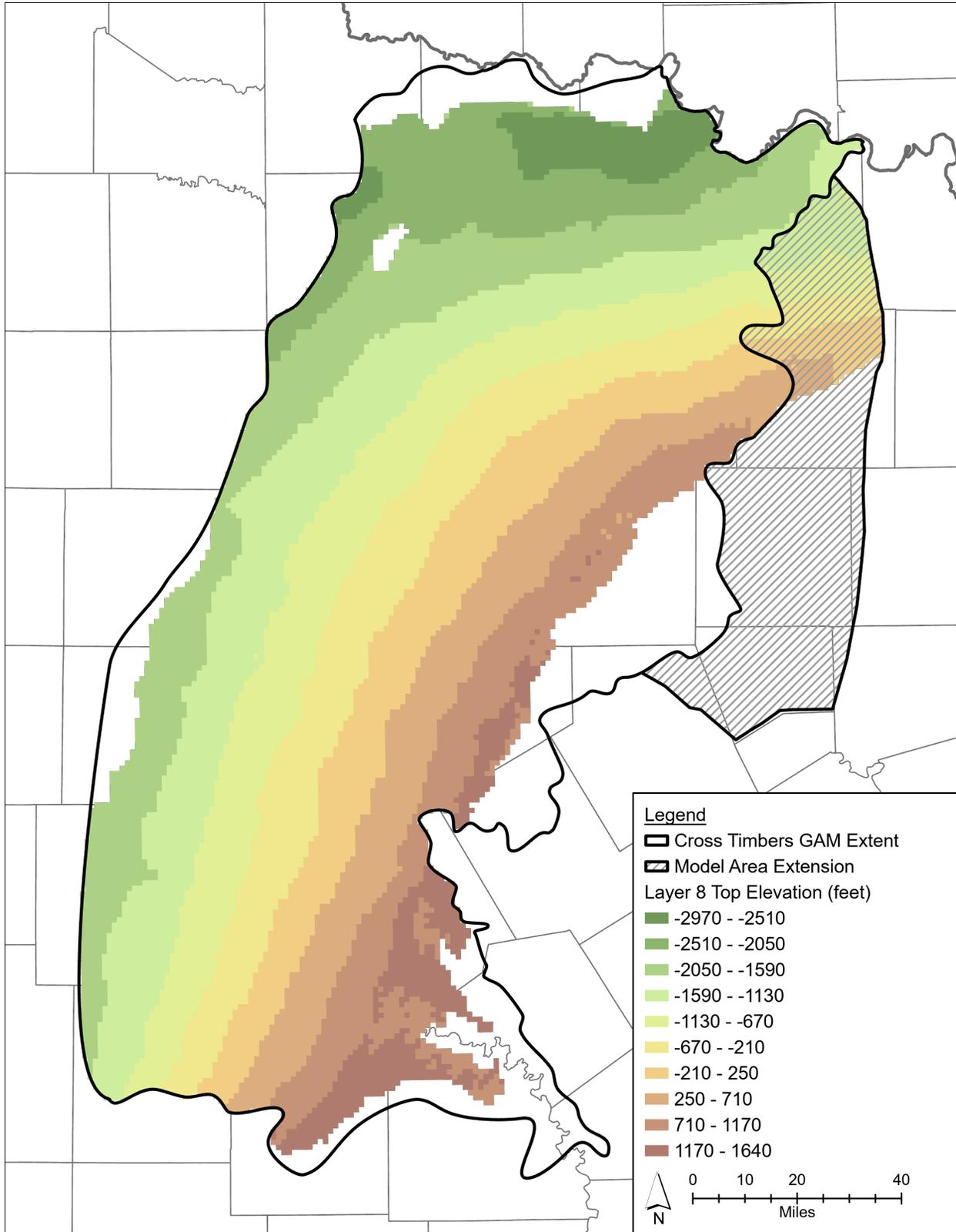
**Figure 3-8. Top elevation of Layer 8, Palo Pinto Formation, non-shaded areas within the GAM Extent represent inactive and/or vertical pass-through cells.**
