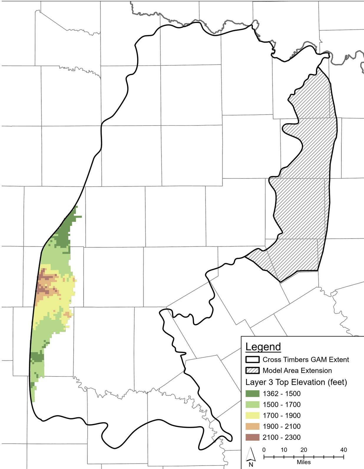
**Figure 3-3. Top elevation of Layer 3, Clear Fork Group, non-shaded areas within the GAM Extent represent inactive and/or vertical pass-through cells.**
