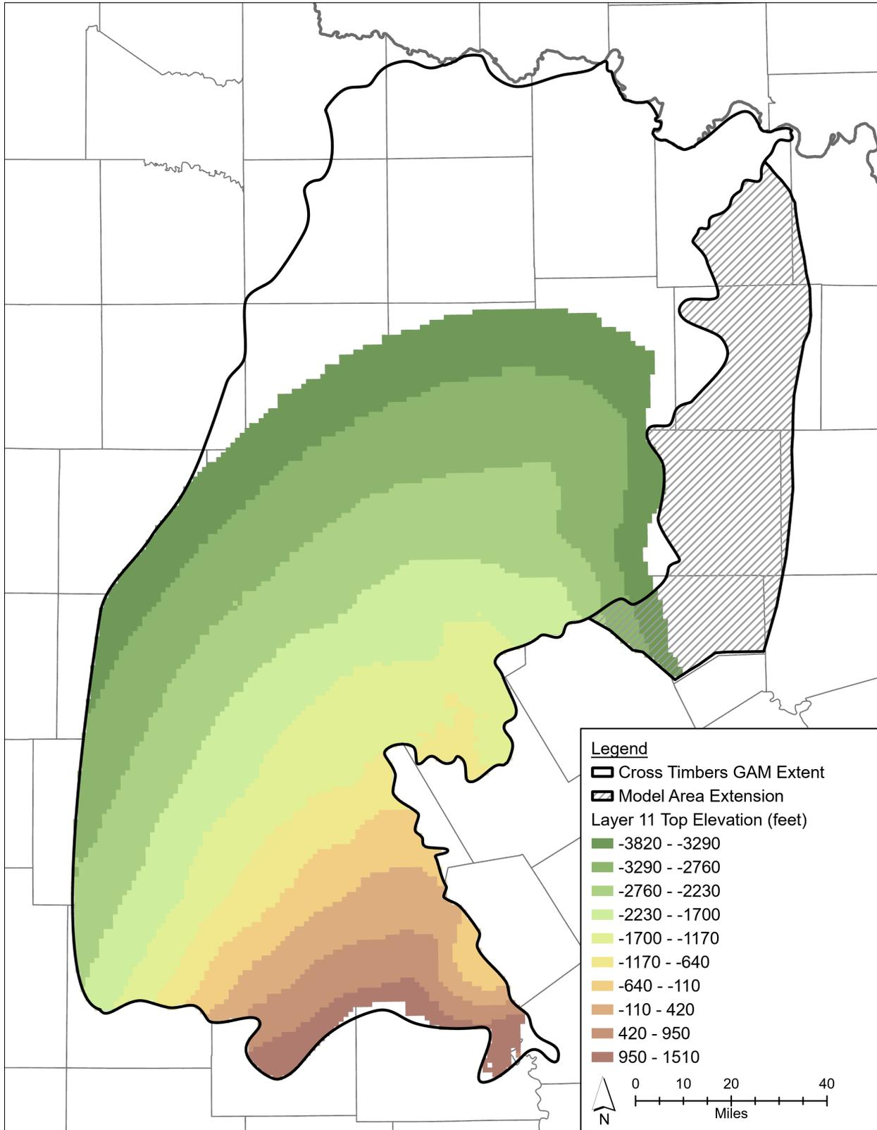
**Figure 3-11. Top elevation of Layer 11, Marble Falls, non-shaded areas within the GAM Extent represent inactive and/or vertical pass-through cells.**
