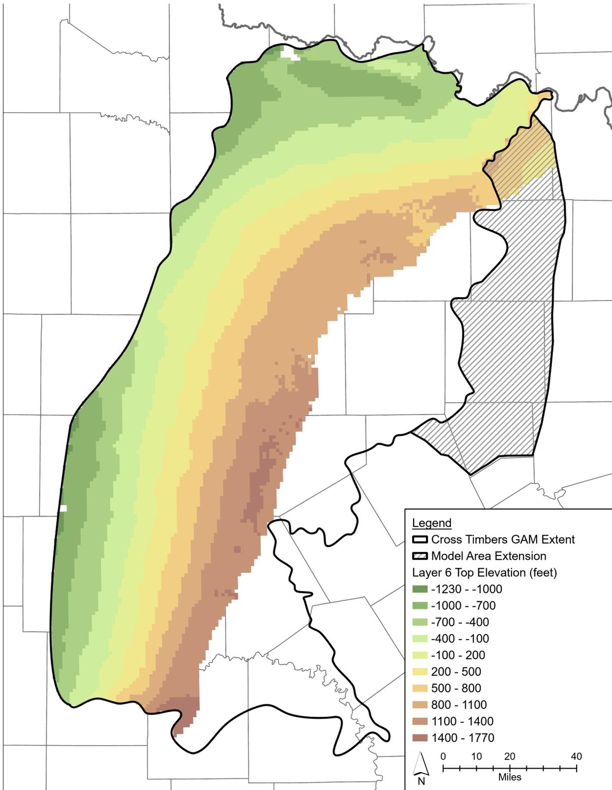
**Figure 3-6. Top elevation of Layer 6, Lower Cisco Group, non-shaded areas within the GAM Extent represent inactive and/or vertical pass-through cells.**
