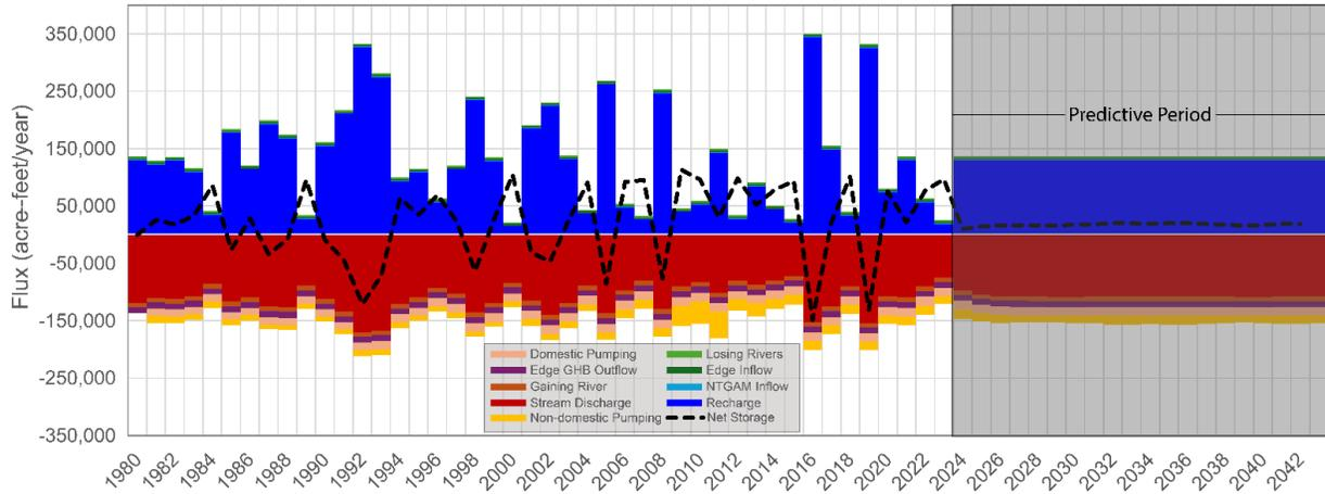
Figure 4-44. Natural inflow and outflow mechanisms to the primary aquifer.
