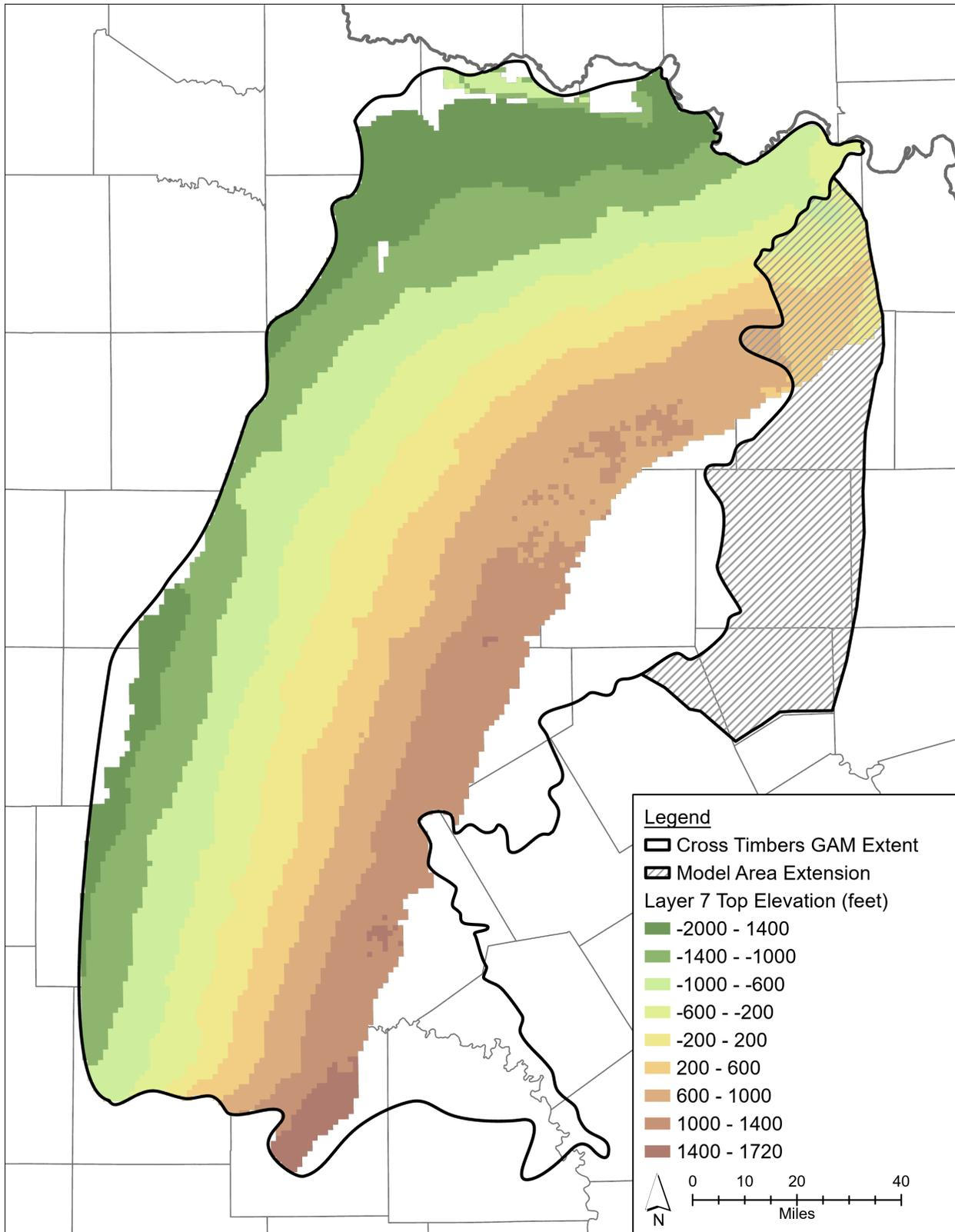
**Figure 3-7.** Top elevation of Layer 7, Canyon Group, non-shaded areas within the GAM Extent represent inactive and/or vertical pass-through cells.
