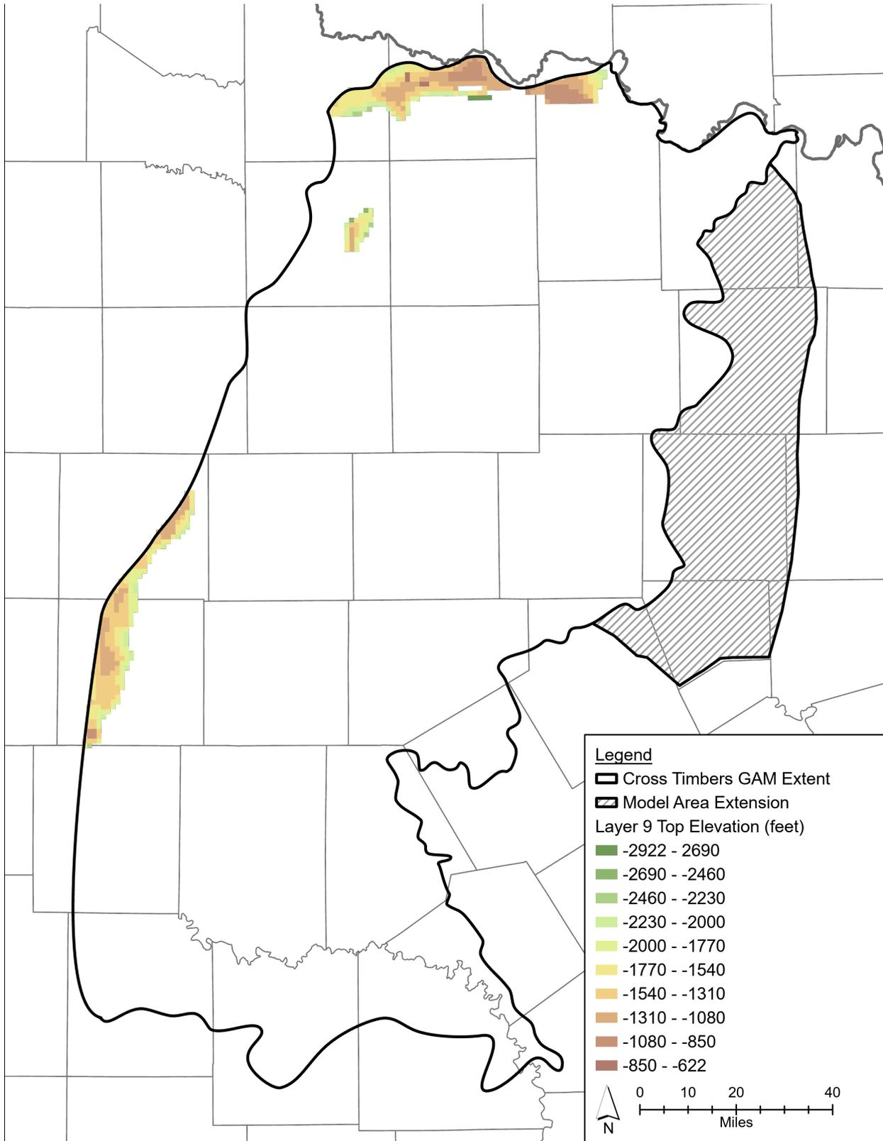
Figure 3-9. Top elevation of Layer 9, Reef Formation, non-shaded areas within the GAM Extent represent inactive and/or vertical pass-through cells.
