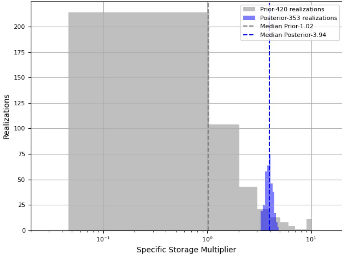
Figure 4-25. Primary aquifer specific storage multiplier prior versus posterior distribution.
