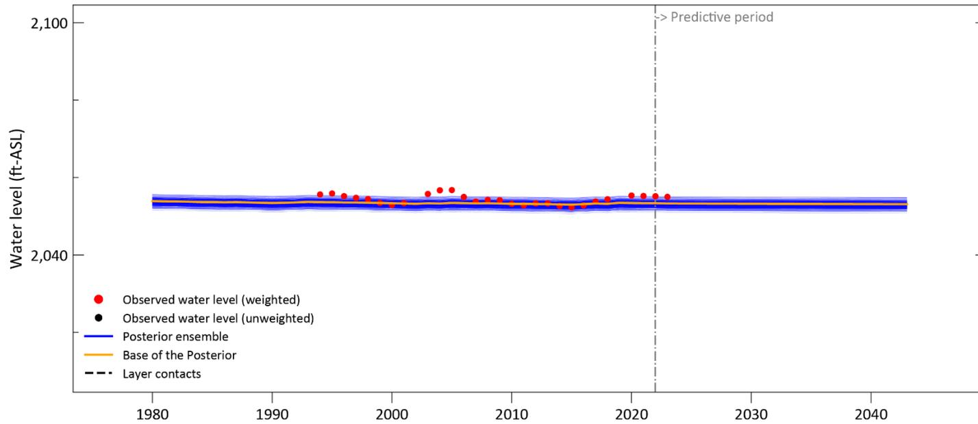
Figure 4-37. Observed (red dots) and simulated (blue lines) groundwater levels in State Well Number 3050801.
