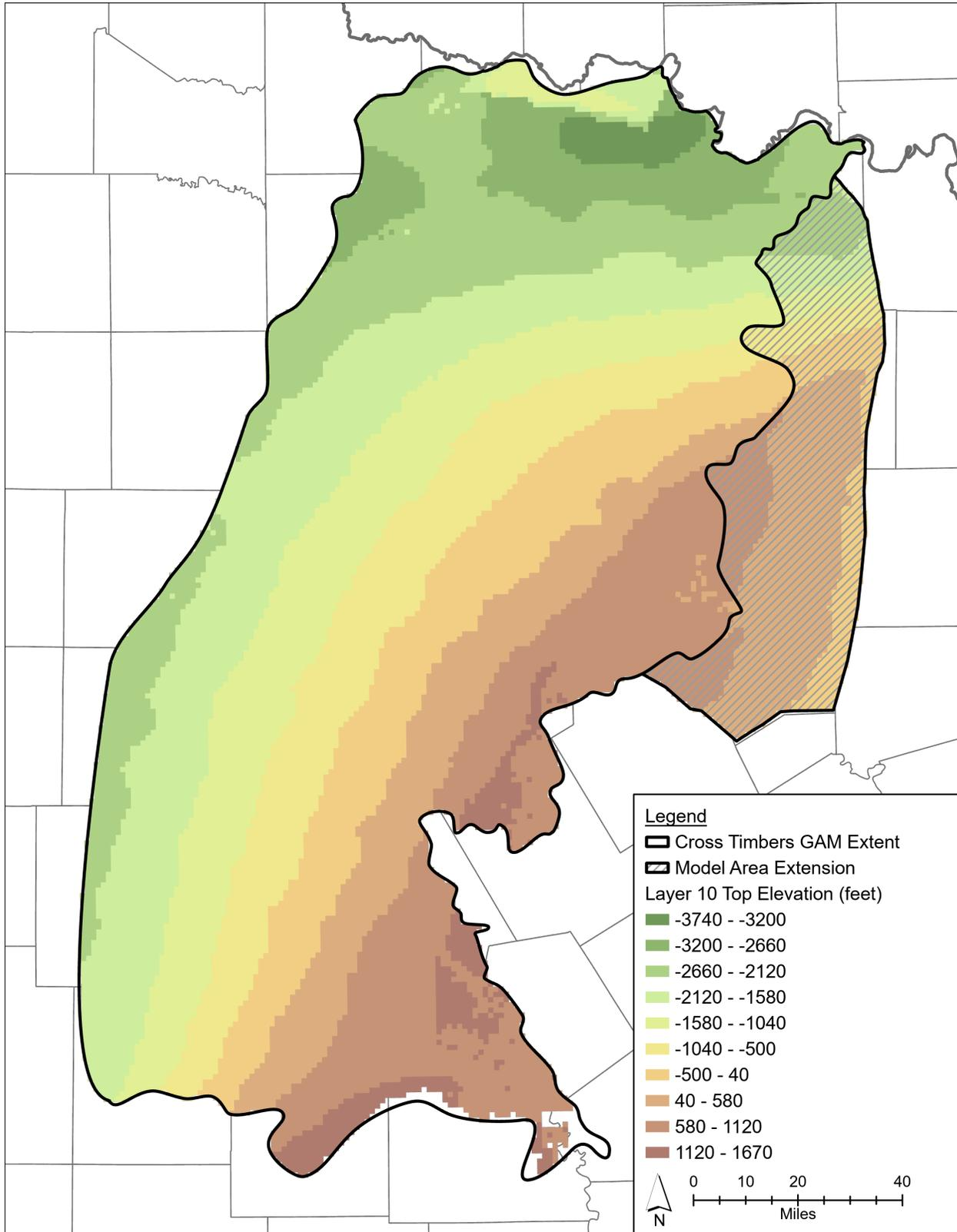
Figure 3-10. Top elevation of Layer 10, Strawn Atoka Group, non-shaded areas within the GAM Extent represent inactive and/or vertical pass-through cells.
