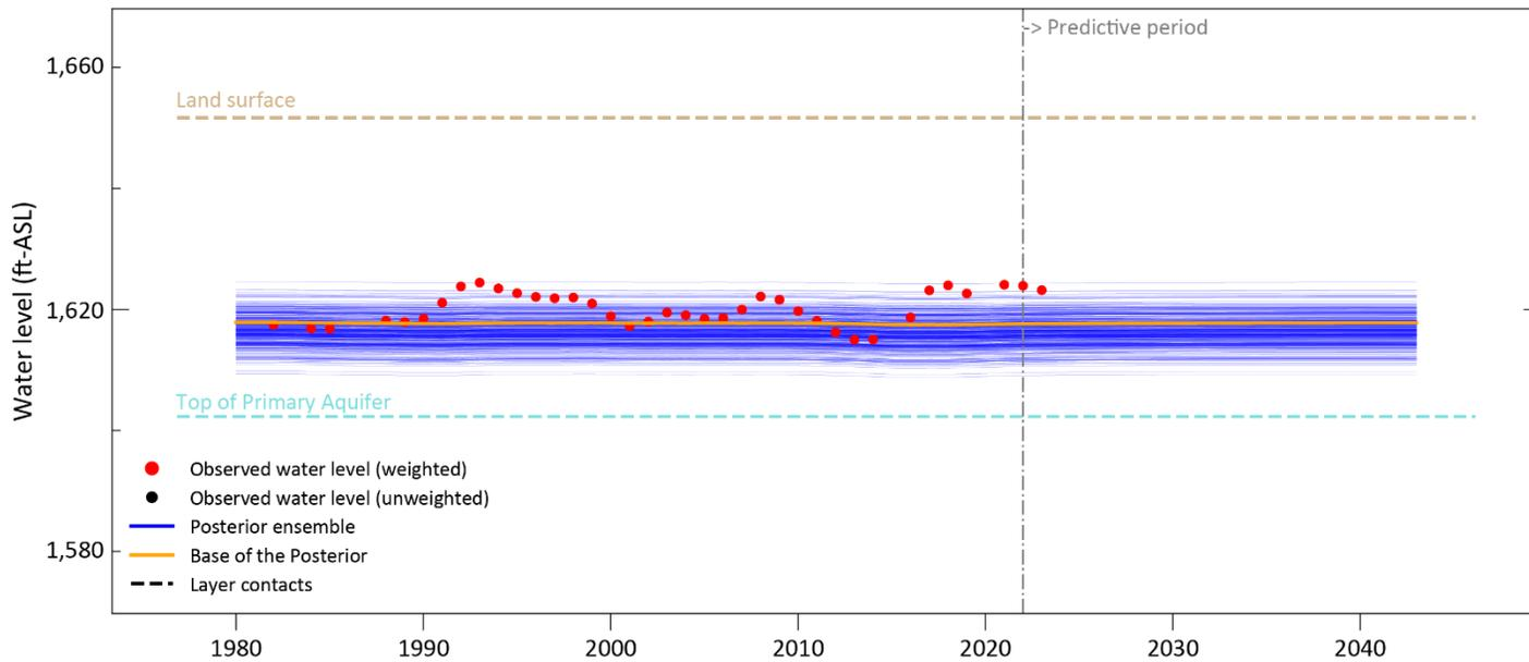
Figure 4-38. Observed (red dots) and simulated (blue lines) groundwater levels in State Well Number 3141401.
