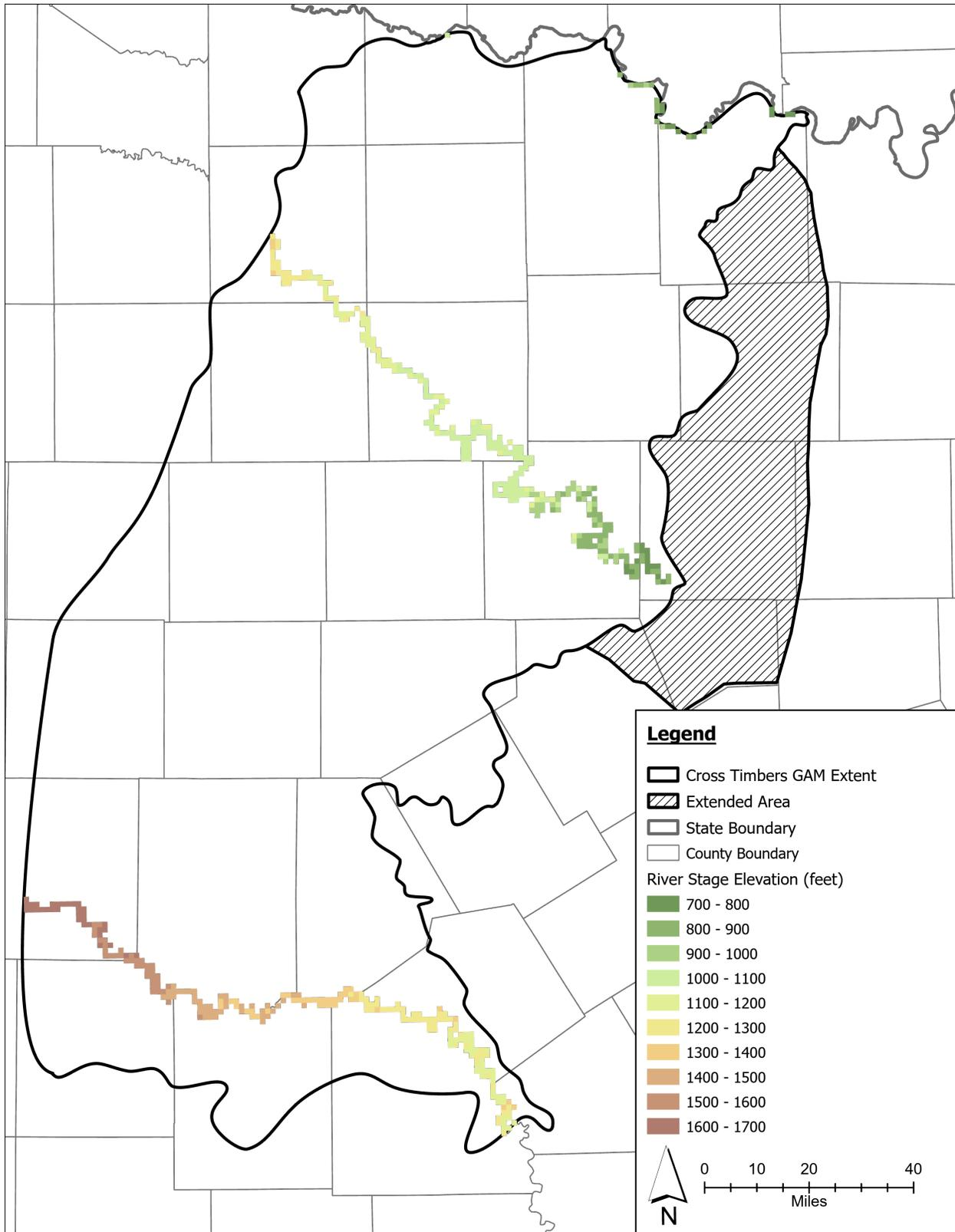
Figure 3-32. River package cells and their stage elevations.
