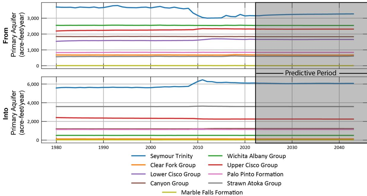
Figure 4-47. Groundwater flow into the primary aquifer and out of the primary aquifer from intersecting aquifers.
