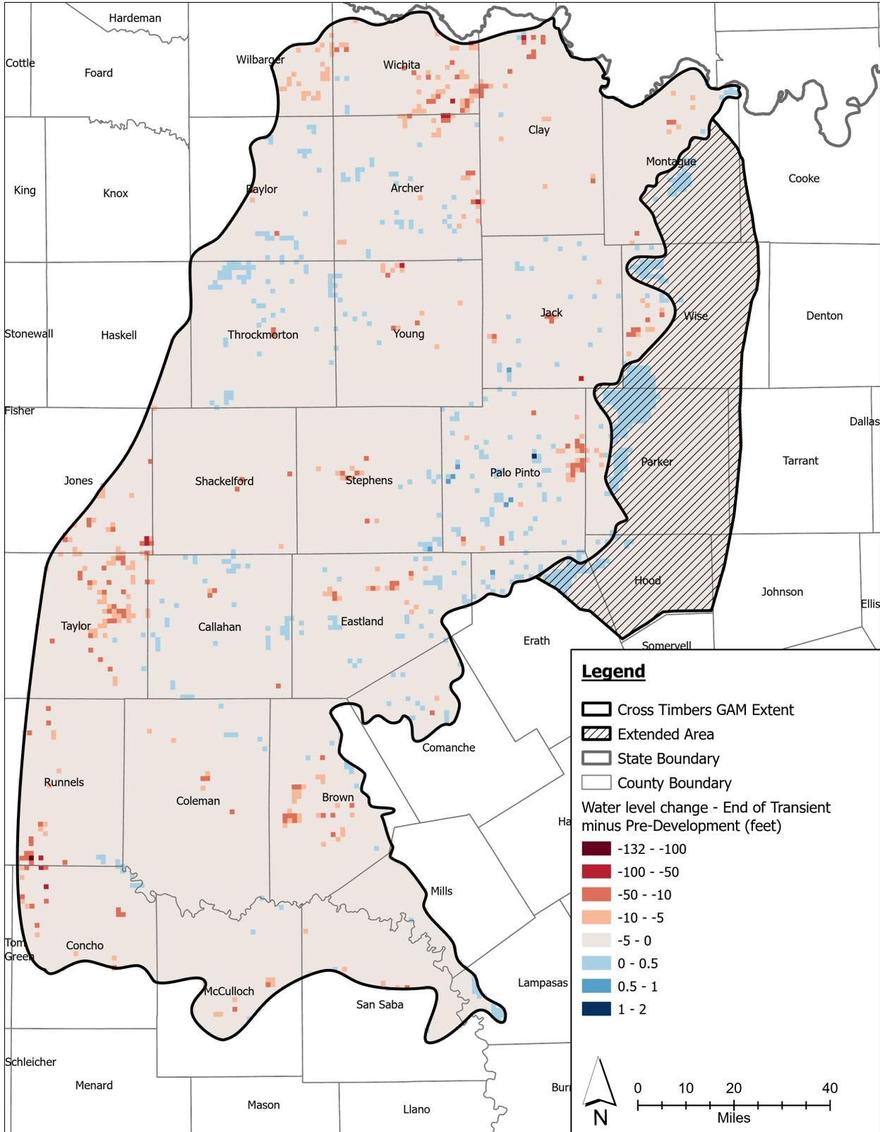
**Figure 4-35. Change in simulated water level between pre-development and the end of the transient period.**
