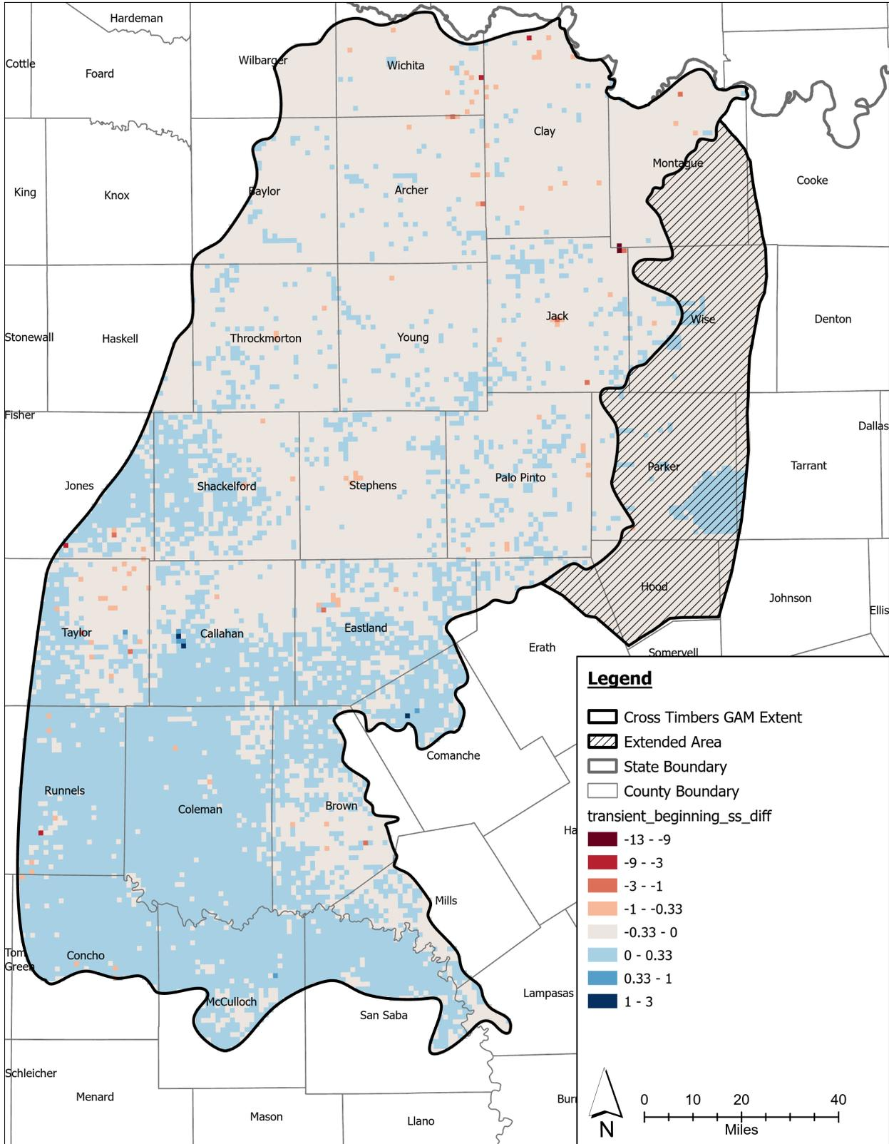
**Figure 4-34. Change in simulated water level between pre-development and the beginning of the transient period.**
