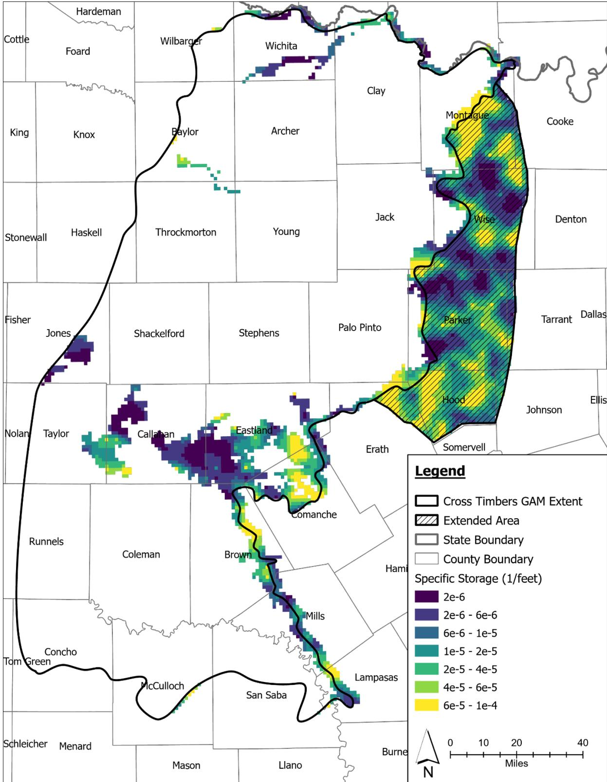
Figure 4-26. Calibrated specific storage for Layer 2.
