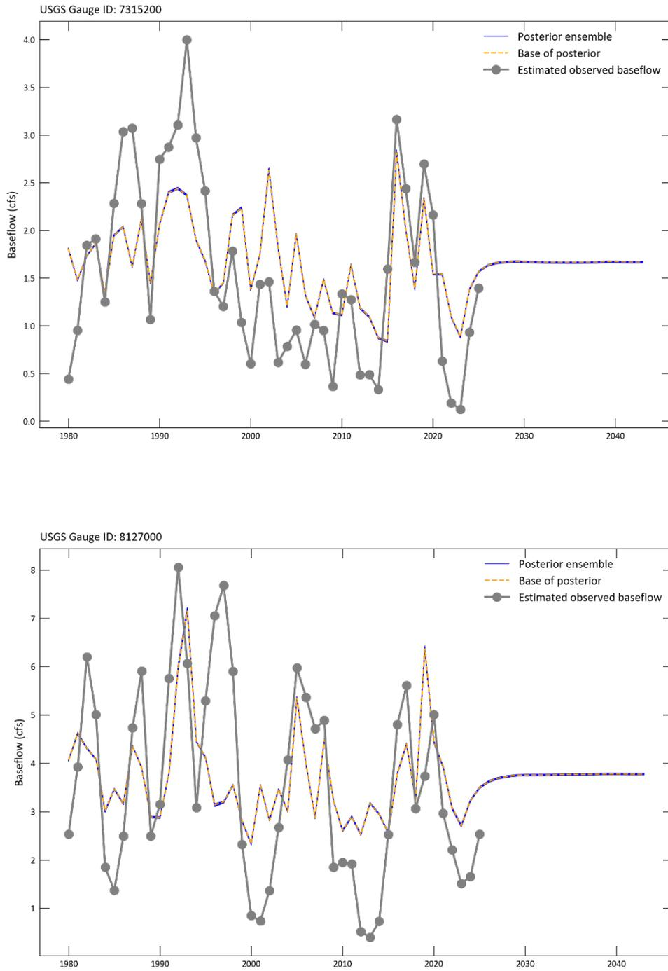
**Figure 4-41. Observed (gray line with dots) and simulated (blue lines) baseflow at United States Geological Survey gauge stations 7315200 and 8127000. The base of the posterior is shown in orange.**
